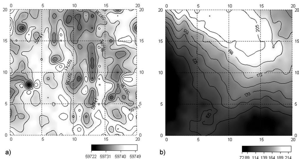
Figure 2. Geophysical survey results with magnetometer data in nanoteslas (a); and electromagnetic induction data for the 9125 Hz frequency in Ec units (b).
